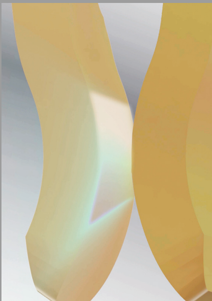
Fig. 4: Contact is established via the smooth surface of the female contact
